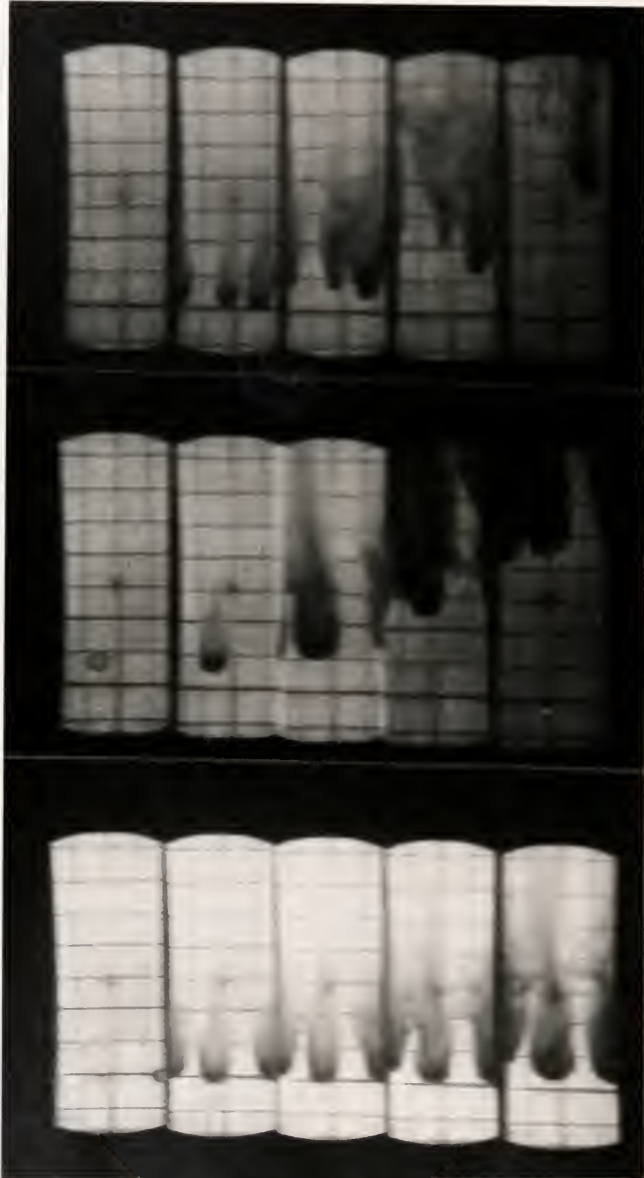
a. FIGURE 5. TYPICAL SHADOW PHOTOGRAPH SEQUENCES: a. D=2.06 mm, M_S=1.84 ; b. D=2.74 mm, M_S=2.01 ; c. D=.985 mm, M_S=1.90 b. c.
